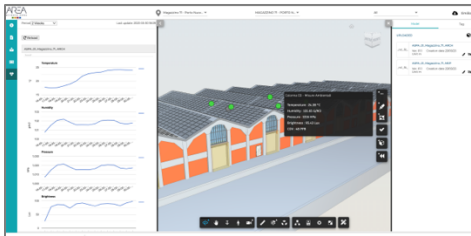
In detail, the measurement trend of the selected sensor. You can see both the detail with mousover on the marker, as well as the detail of the trend graphs by selecting the marker.
